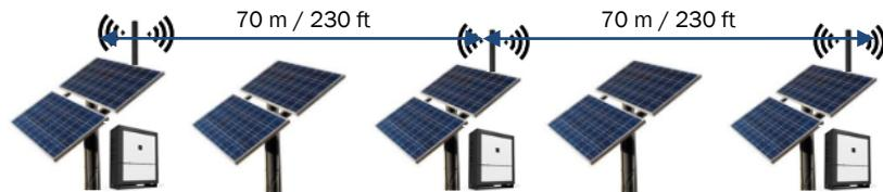
Ingeteam states that the *Wi-Fi Mesh* network cannot have more than three hops. Thus, the maximum allowed distance in a *Mesh-Cell* between an inverter and the most distant *MeshBridge* is 210 meters / 690 feet.
