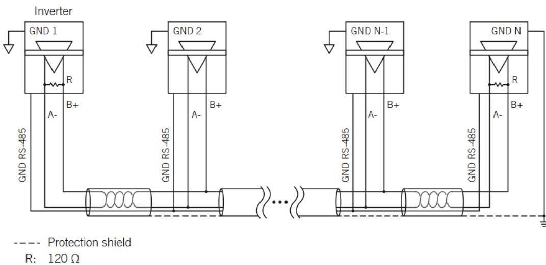
The installation of the following example includes several inverters connected in the bus and a measurement converter to which a local PC is connected.
